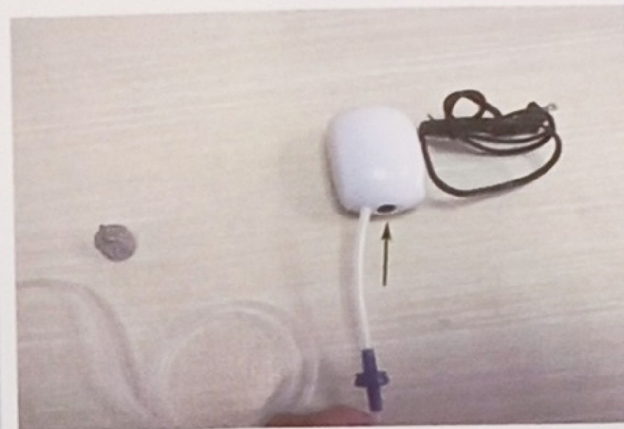
3. Connecting the silicone hose with air pump.
