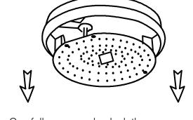
Carefully press and unlock the screw on the led hinged tray and hold the tray at an upward 90Degree position. Hold the product upside down.
