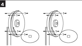
Hold the product in place, mark & drill the holes into the wall and nail the alligator into the hole. Feed the supply cable into the luminaire through the cable entry hole
